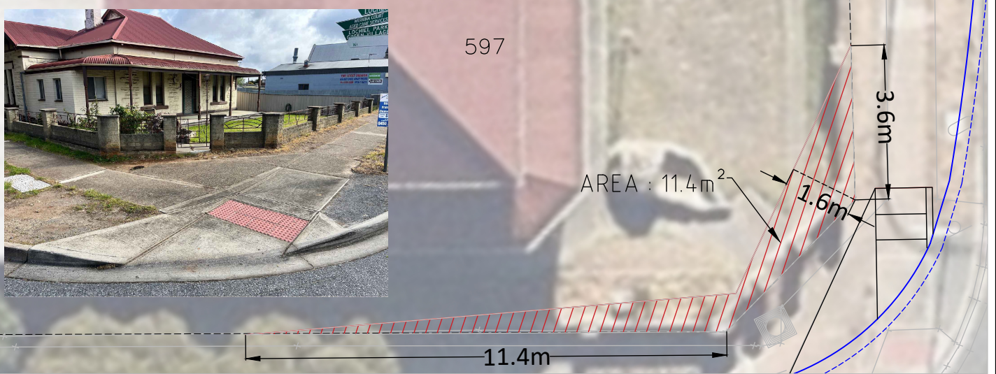
ENLARGEMENT - LAND ACQUISITION SCALE: 1:125 (A3)
